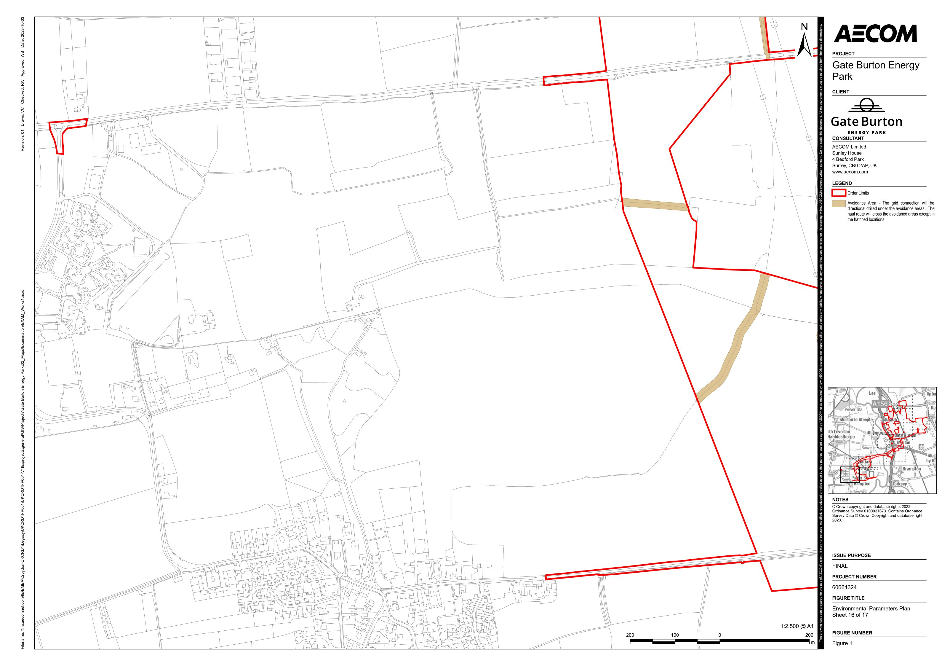
Avoidance Area - The grid connection will be directional drilled under the avoidance areas. The haul route will cross the avoidance areas except in the hatched locations
